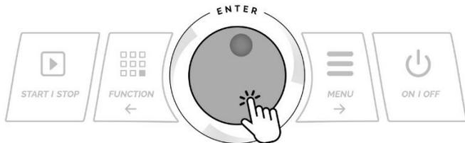
4. Rotate the dial to select the direction. Press on the dial-knob to put the cross-head in motion. Press on the dial or the START / STOP button to stop the cross-head.
