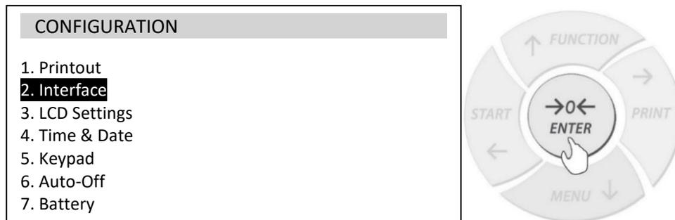
3. To enable the Wireless transmitter, select Bluetooth and press the Enter key. Select Status and use the navigation keys to select ON.
